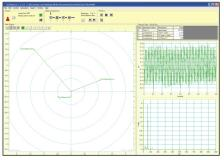
eZ-Balance™ automatically computes the optimal balance weight and location
