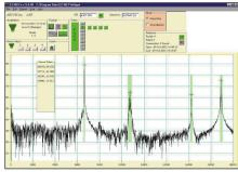
eZ-NDT™ compares the acoustic signature of known-good objects to test objects, and determines whether the test object is good
